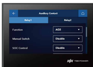
Generator AGS Control Setting
